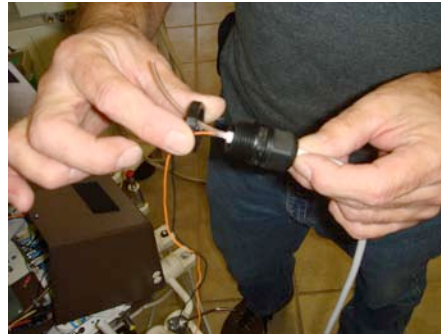
Fig.8 Remove black plastic nut on new ultrasonic cord
