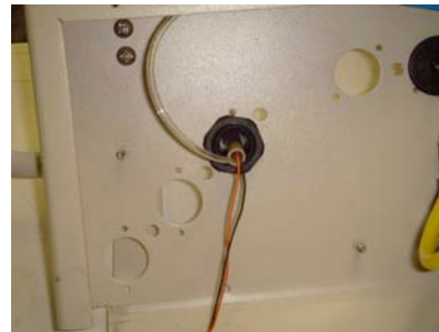
Fig.2 Locate bulkhead inside cart
