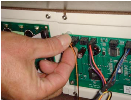
Fig.3 Pinch Black Plastic fitting to disconnect
