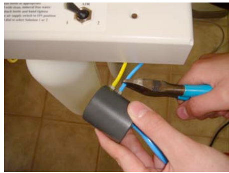
Fig. 6 Clip tubing at barb
